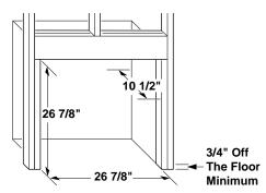
Figure 8 - Rough Opening for Installing in Wall
